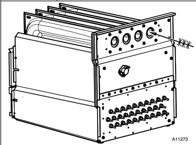
**NOTE:** After cleaning, inspect the heat exchangers to ensure they are free of all foreign objects that may restrict flow of combustion products.
