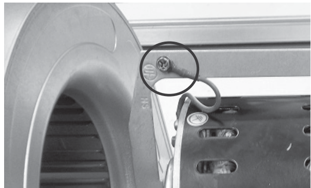
Figure 12 – Disconnect Ground Wire
