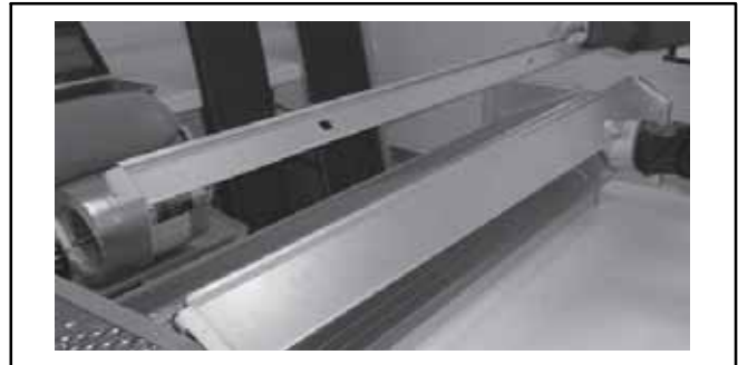
Figure 22 – Insulation Support Brackets
