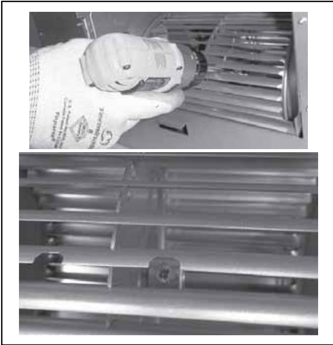
Figure 15 – Loosen Blower Set Screw
