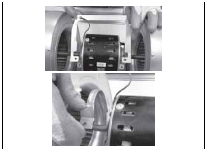
Figure 12 – Remove Grounding Bracket
