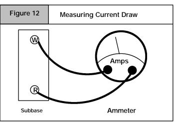
The best method to obtain the required setting for the heat anticipator, is to measure the actual current draw in the control circuit ("W") using a low range (0–2.0 Amps) Ammeter. (See **Figure 12**) After measuring the current draw, simply set the heat anticipator to match that value.
