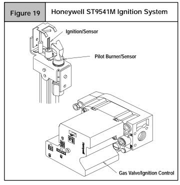
The system consists basically of only two (2) components. The Ignition System Control and the Pilot Hardware. The operate on Two (2) 24 volt power circuits received from the ST9160B Fan Timer/Furnace Control. One is the power supply to the ignitor, the second is to activate the ignition sequence.
