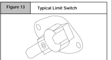
To verify this, the cut-out (opening) point of the switch should be checked (using a thermocouple type thermometer connected to the face of the switch) as follows:
