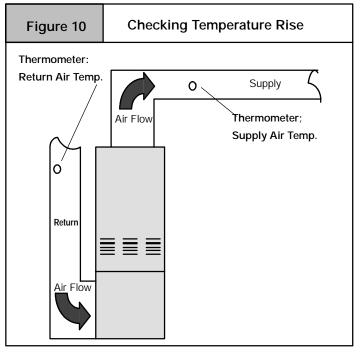
The furnace is designed to operate within a certain specified range of temperature rise.
