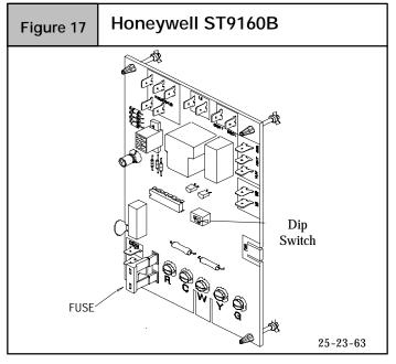
The Honeywell ST9160B Electronic Fan Timer/Furnace Control contains NO USER SERVICEABLE COM-PONENTS. It is, as its name implies, a fan timer and a furnace control of sorts. In addition to controlling the fan operation for heating, it also takes the place of the blower relay, the combustion air relay and/or the system relay.
