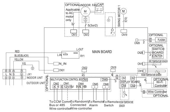
Fig. 4 — Wiring Diagram Sizes (115V)
