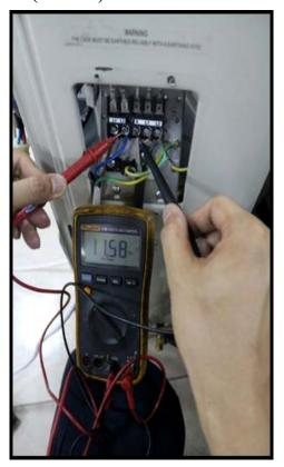
Fig. 23 — Test the DC Voltage
