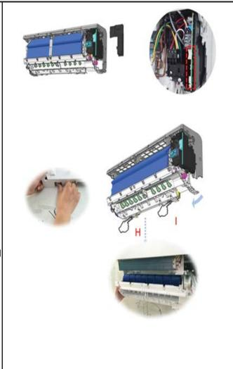
Front panel How to remove the evaporator assembly Caution: Because the 24K indoor unit is relatively large and heavy, a minimum of two persons are required to implement the following steps. 1) Remove the electric control box. 2) Remove the chassis assembly. 3) Unfold the Pipe clamp board (C), remove screws A and B. 4) Pull out the evaporator.
