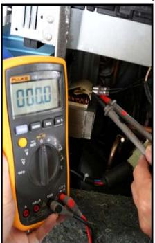
Fig. 24 — Test the Reactor Resistance
