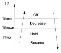
Fig. 18 - Evaporator Coil Temperature Protection
