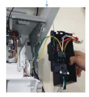
Front panel How to remove the chasis assembly Caution: Because the 24K indoor unit is relatively large and heavy, a minimum of two persons are required to implement the following steps. 1) Remove the left and right pipe cover. 2) Remove the 5 screws A,B,C,D,E remove support parts F and G. 3) Open the E-box, to unhook the fan motor and louver motor connectors from the PCB.
