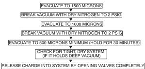
Fig. 10 - Triple Evacuation Method
