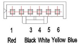
Fig. 25 - Motor Connector
