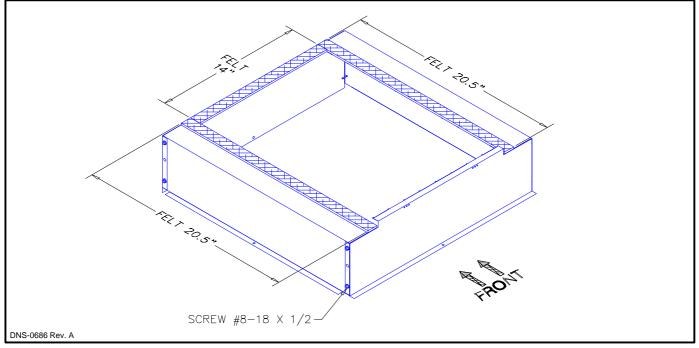
2- Fix the OCA and "B15" series cased coil on the furnace as shown on drawing.
