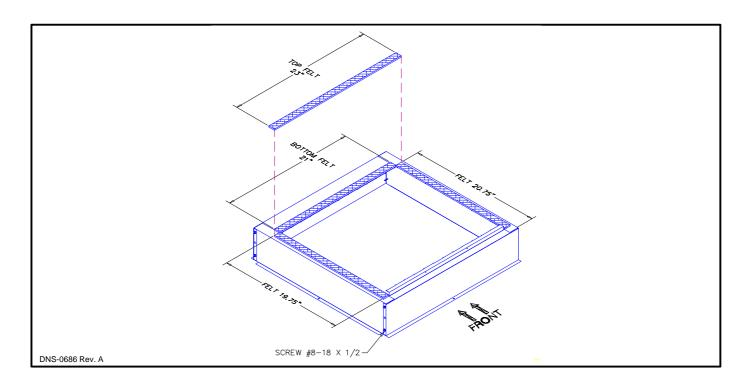
2- Fix the OCA and "J22" series cased coil on the furnace as shown on drawing.
