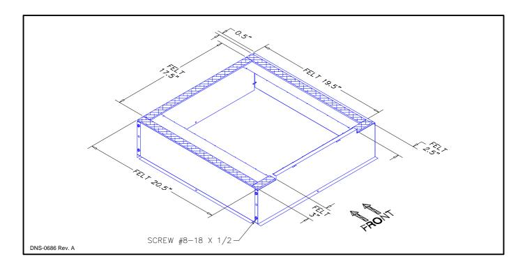
2- Fix the OCA and "F19" series cased coil on the furnace as shown on drawing.
