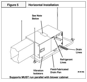
**NOTE:** If increased structural strength is needed in the horizontal position, use field supplied two connecting plates in place of the tabs on the bottom of the blower.
