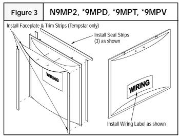
1. Place one Wiring Label on the inside of the door.
