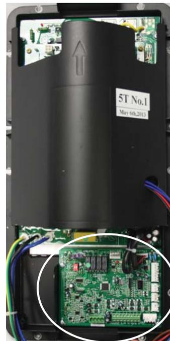
Figure 22 – Panneau de commande AOC (Application Operational Control)
