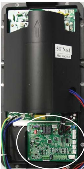
**Figure 17 – Panneau de commande AOC (Application Operational Control)**
