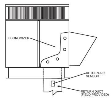
Fig. 15 - Return Air Enthalpy Sensor Mounting Location
