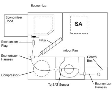
Fig. 9 - Routing Harness (Top View)
