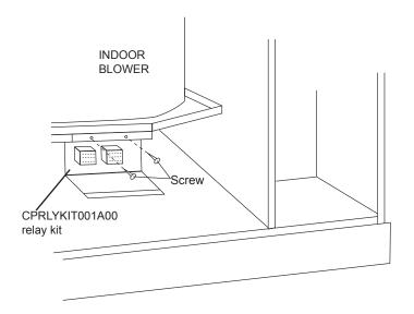
Fig. 12 - Relay Kit Installation
