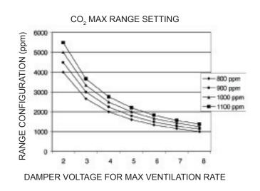
Fig. 18 - CO<sub>2</sub> Sensor Maximum Range Setting
