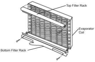
Fig. 1B - Filter Rack Installation (Straight Coil)
