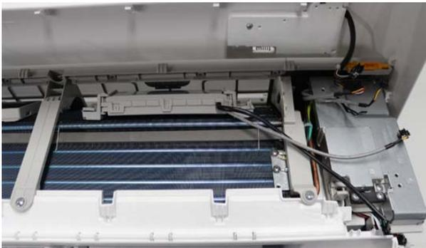
**Fig. 32 — Connect the multi-function board**
