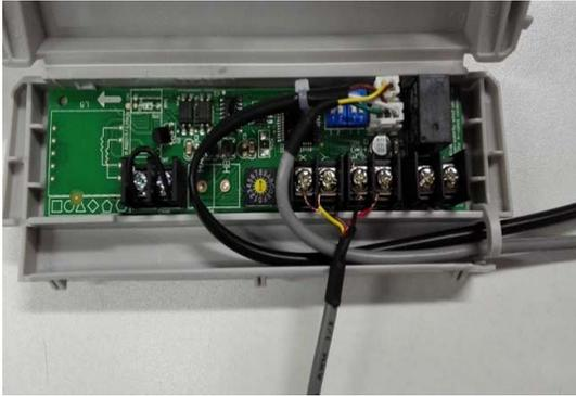
**Fig. 30 — Connect the cable to the board**
