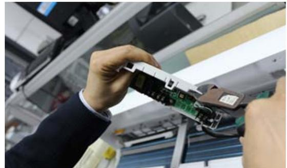
**Fig. 28 — Cut a hole on the multi-function board**
