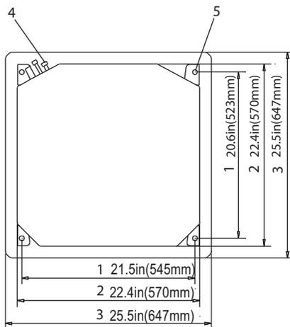
**Fig. 4 – Drilling Holes**
