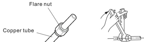
**Fig. 31 – Tighten the Flare Nut**
