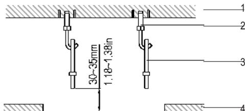
**Fig. 7 – Installation Clearances**
