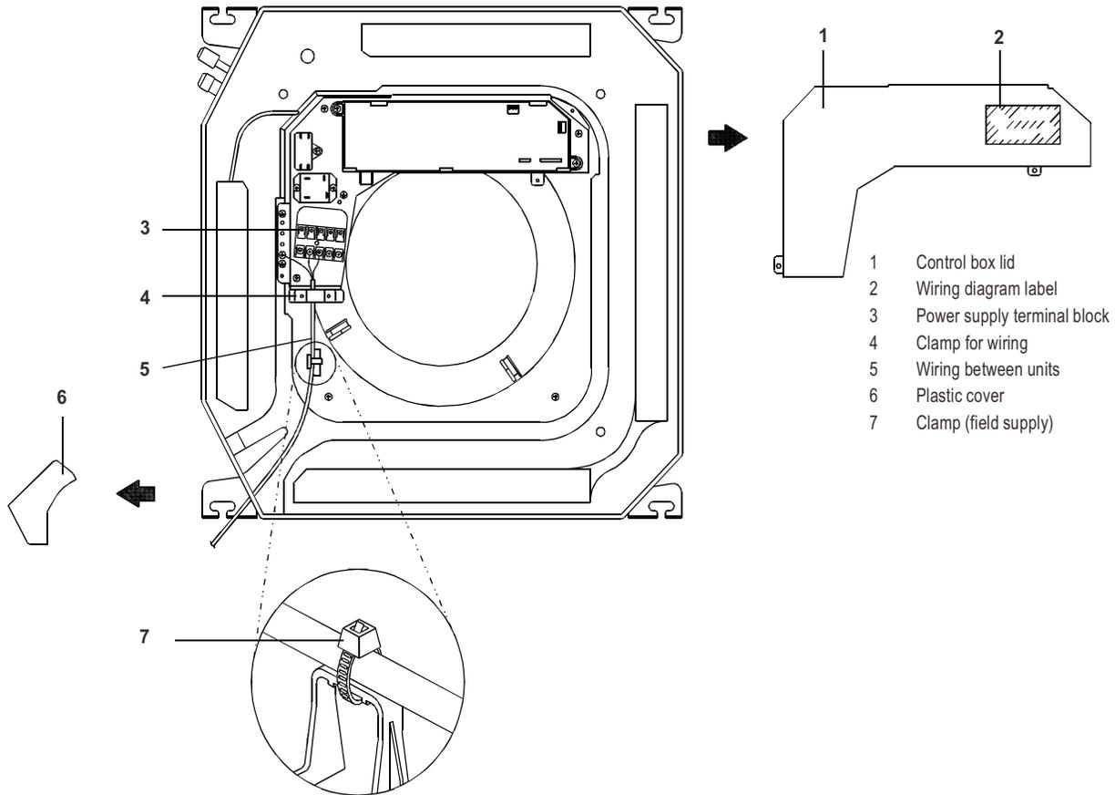
**Fig. 16 – Wiring/Control Box**
