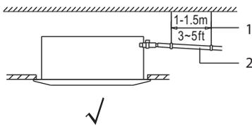
Fig. 10 – Drain Piping Installation
