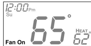
**Fan On** indicates constant fan operation. This feature is active even if the thermostat is set to **Off**.
