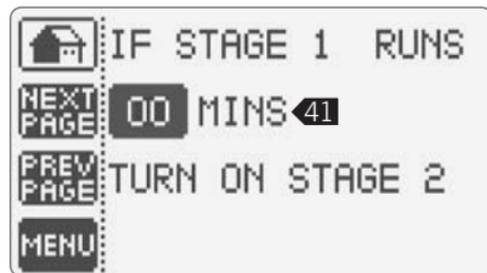
**41** Specify X minutes for which stage 1 will function until stage 2 is activated to help raise (or cool) temperature (if the temperature set point is not reached). This function avoids excess compressor wear in the case where the necessary temperature set point is not met (see [37](#), [38](#) & [39](#)). Set to "00" to disable.
