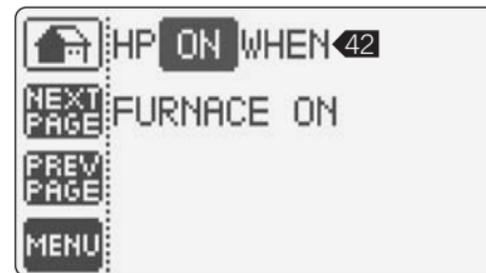
**42** HP "ON" when Furnace On: Heat Pump and Furnace can operate together when 2nd stage furnace is required.
