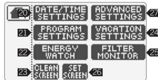
**23** This function allows you to wipe and clean the screen with a dampened cloth with out accidentally changing any of the settings; it place the thermostat screen in a sleep mode for 15 seconds.
