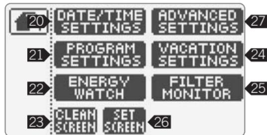
**25** Displays filter usage in days and resets filter timer.
