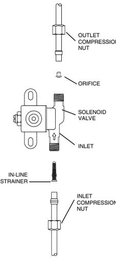
1. Disconnect electrical power to the furnace and shut off water supply.
