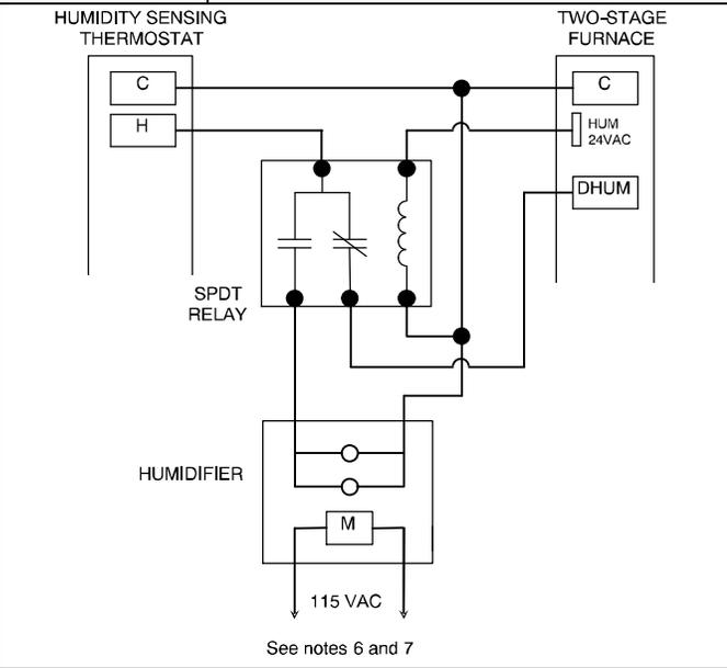
**Figure 23 Two-Stage Furnace and Humidifier Only**
