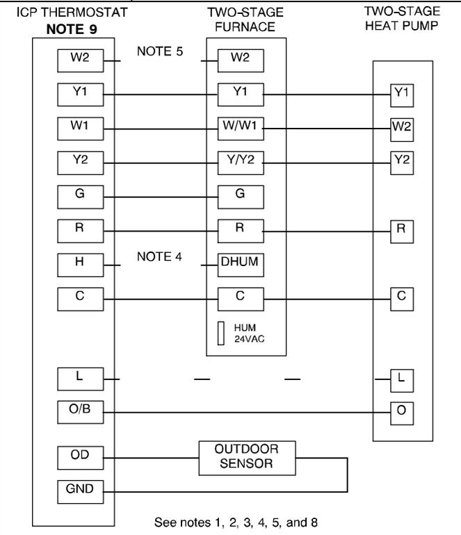
**Figure 22 HP with Two-Stage Furnace, Humidifier, and Dehumidification**
