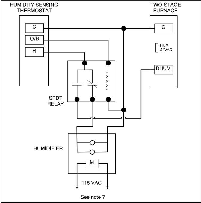
**Figure 21 AC with Two-Stage Furnace, Humidifier, and Dehumidification**
