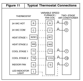
**NOTE:** Optimal comfort, efficiency, and reliability will only be achieved when the indoor airflow is properly set for both low-stage and high-stage operation.
