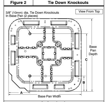
Inches (mm) Tie Down **Base Pan** Minimum Knockouts Width x Mounting Pad Depth Α В С Dimensions 23 x 23 7–3/4 4-7/16 23 x 23 18 (584 x 584) (197) (113) (457) (584 x 584) 25-11/16 x 9-1/16 4-7/16 21 - 1/426 x 26 25-11/16 (230) (113)(540) (660 x 660) (652 x 652) 31-1/8 x 31-1/8 9-1/16 6-1/2 24-5/8 31–1/2 x 31–1/2 (791 x 791) (230) (165)(625)(800 x 800)
