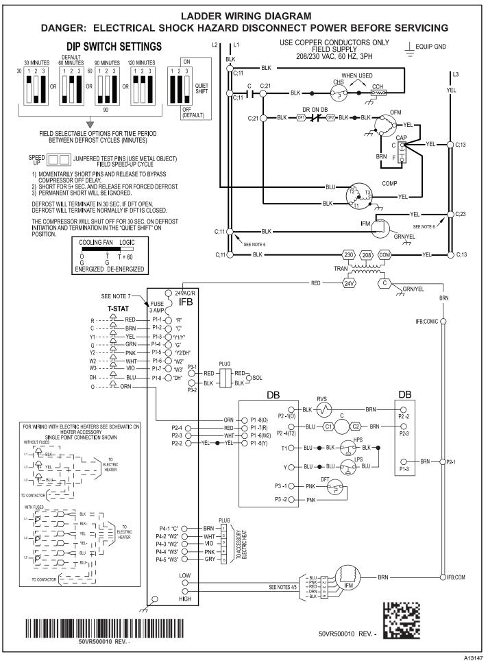
Figure 16 Cont. - Ladder Wiring Diagram 208/230-3-60
