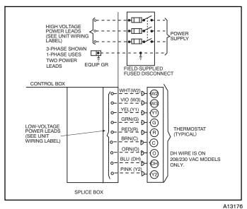
Figure 10 - High- and Control-Voltage Connections
