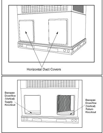
Figure 9 - Supply and Return Duct Opening
