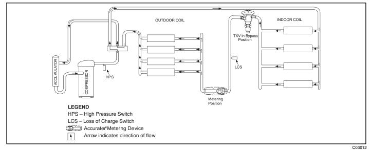
Figure 13 - Typical Heat Pump Operation, Heating Mode
