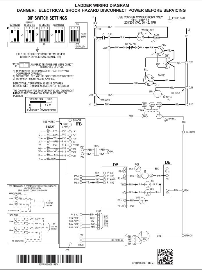
Figure 15 Cont. - Ladder Wiring Diagram 208/230-1-60
