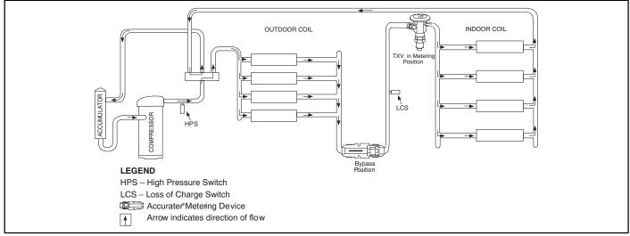
Figure 14 - Typical Heat Pump Operation, Cooling Mode
