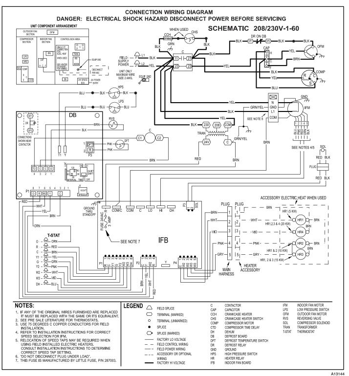
Figure 15 - Connection Wiring Diagram 208/230-1-60
