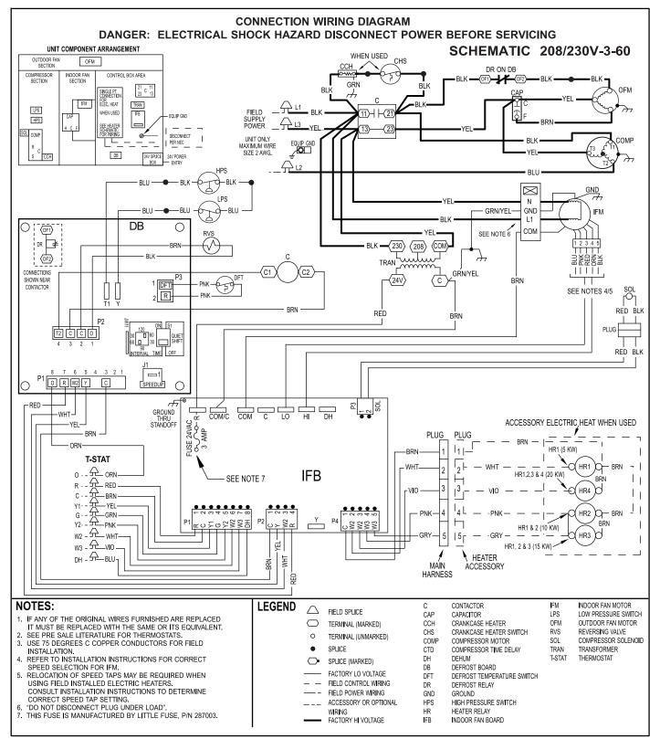
Figure 16 - Connection Wiring Diagram 208/230-3-60
