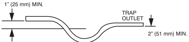
Condensate Trap (Using Tubing)
