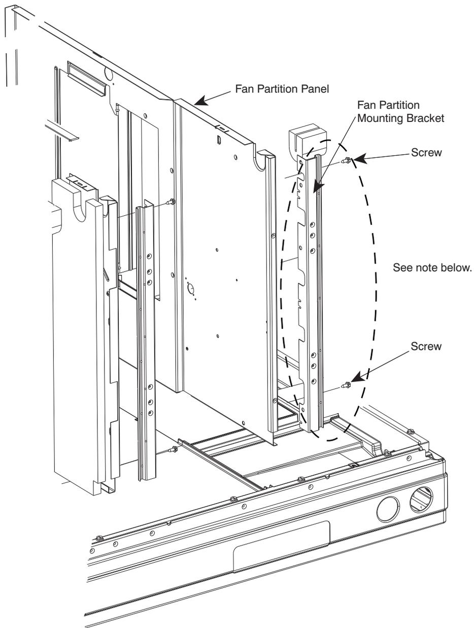
NOTE: The fan partition bracket may be removed for easier access to the burner assembly. The bracket may be removed by removing 2 screws on the control side and sliding the bracket forward, bottom first.
