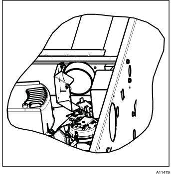
Figure 6 – Rain Shield Installation
