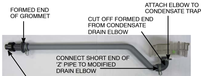
Figure 15 Drain Trap Connection and Routing
