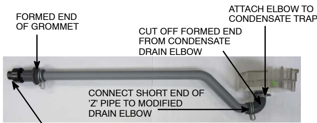
Figure 17 Drain Trap Connection and Routing
