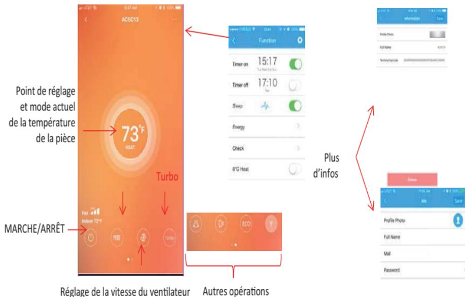
**Figure 15 – Interface principale de commande**
